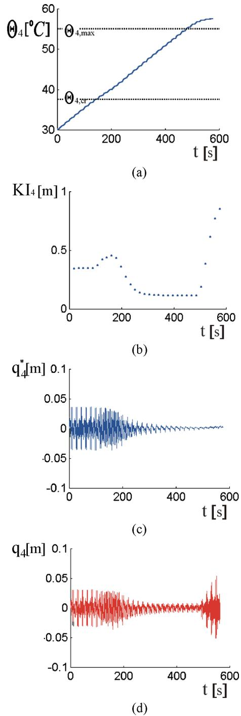
Fig. 7. Behavior of joint 4: (a) joint fatigue  $\Theta_4(t)$ , (b) joint involvement  $KI_4(t)$ , (c) reference motion  $q_4^*(t)$ , and (d) realized motion  $q_4(t)$ .
